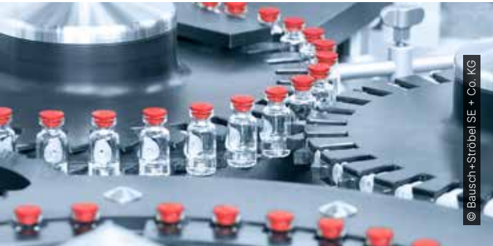
Particularly gentle, low-particle object transport in which the glass vials are held in a vacuum.
